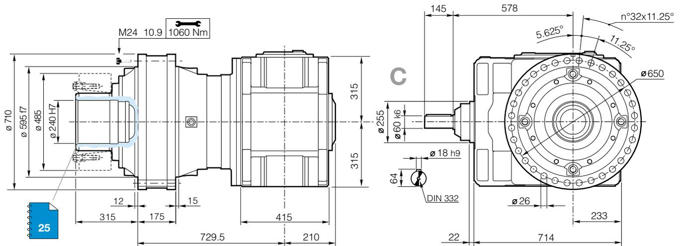
Output male cylindrical and splined shafts available on request.
