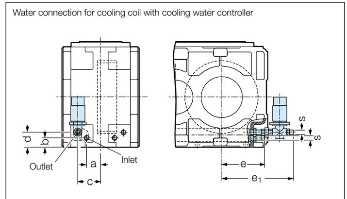
Cooling coil placed adjacent to the final gear wheel. For the gear wheel position see the dimension sheets
